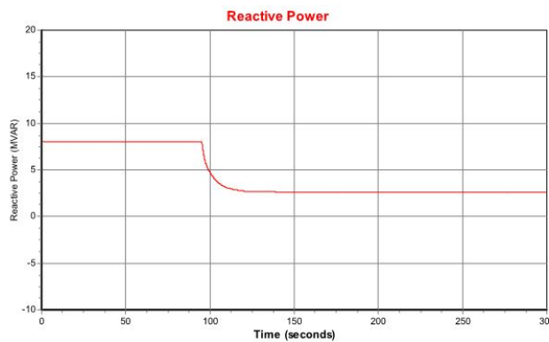
Fig. 10: Simulated reactive power response to plant step change in voltage
