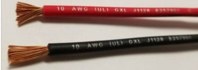
Fig. 6. AWG wire verification on the insulation.
