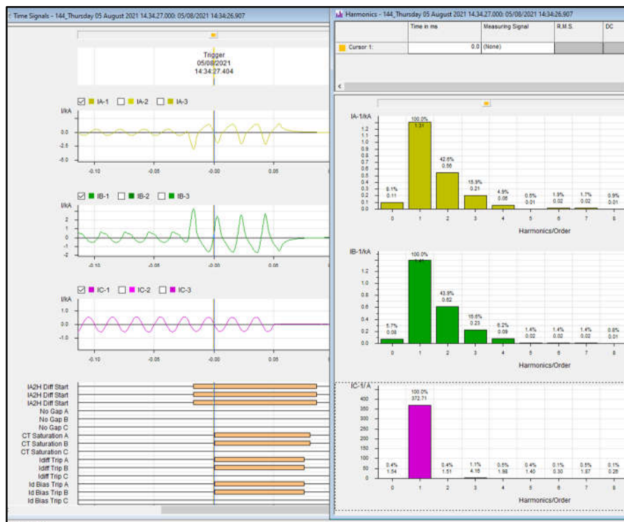
Figure 40 CT saturation during an internal fault condition
