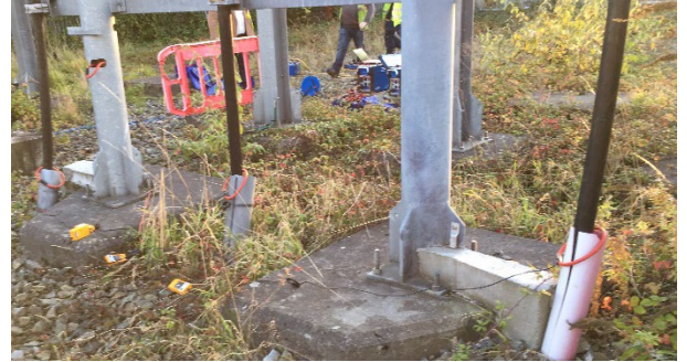
Fig. 12. Primary measurement of I_p with 4 Rogowski coils
